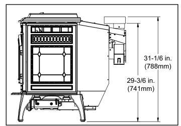
Figure 8.2 - Side View with Top Vent Adapter and
